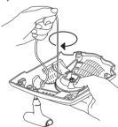
Stretch the line with the handle. Move your thumb and release the line. See the figure below.
